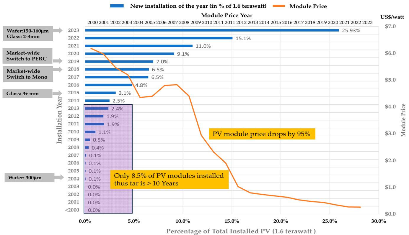
Figure 1. Global PV installation, module price, and technical development 2000–2023.
