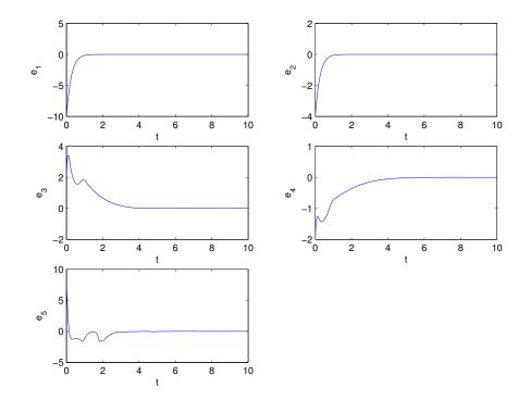
Figure 4. The time response of error states with controllers as in Equation (16).
