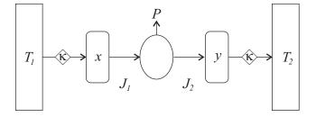
The parameter R takes values within the interval  $0 < R \leq 1$  (R = 1 corresponds to the endoreversible limit), and it can be seen as a measure of the departure from the endoreversible regime when R < 1 [18,23]. If we assume that the heat flows from  $T_1$  to  $\bar{x}$  and from  $\bar{y}$  to  $T_2$  are of the Newton type, then:
