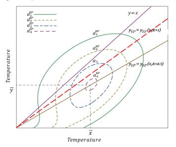
**Figure 3.** Qualitative plots of level curves of the Lyapunov function  $V_{EF}(x, y)$  for the non-endoreversible case with R = 0.5. Here, the constant was chosen satisfying  $\alpha_4^{EF} < \alpha_3^{EF} < \alpha_2^{EF} < \alpha_1^{EF}$ . As a guide, we also show the lines  $y_{EF} = y_{EF}(x)$  and  $y_{EF} = y_{EF}(x, R)$ , which represent the endoreversible (R = 1) and the non-endoreversible (R = 0.5) limits, respectively.
