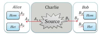
**Figure 1.** Schematic of the continuous-variable version of quantum key distribution (CV-QKD) protocols with an untrusted source. Both the entangled Gaussian source and the quantum channels are fully controlled by Eve. However, Eve has no access to the apparatuses in Alice's and Bob's stations. Alice and Bob can perform either homodyne (Hom) or heterodyne (Het) detection, using either direct or reverse reconciliation.
