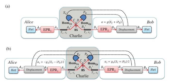
**Figure 2.** (a) Entanglement-based CV-QKD protocol with an untrusted relay where the displacement operator is placed at Bob's side. (b) Entanglement-based scheme where the displacement operator is placed at both Alice's and Bob's sides.
