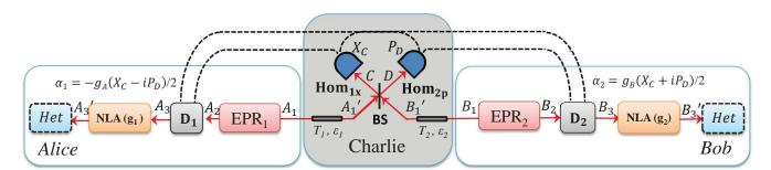
**Figure 6.** Entanglement-based scheme of the modified CV-QKD protocol with an untrusted relay, where a displacement operator D is placed at both Alice's and Bob's sides and the two NLAs are placed before the measurement devices.
