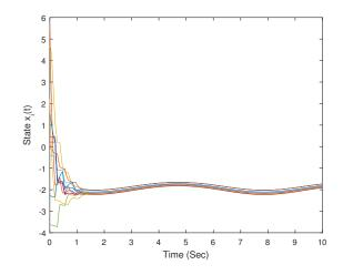
**Figure 2.** State  $x_i(t)$  under the state-controlled switching topologies with a threshold  $\omega = 0.1$ .
