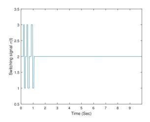
**Figure 3.** The state-controlled switching signal  $\sigma(t)$  with a threshold  $\omega = 0.1$ .
