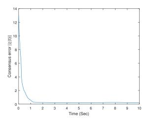
**Figure 4.** Consensus error  $||\xi(t)||$  under the state-controlled switching topologies with a threshold  $\omega = 0.1$ .
