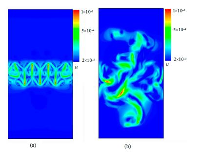
**Figure 3.** Snapshots of the velocity fields with time evolution obtained at times (**a**)  $t/\tau = 1.2$ , and (**b**)  $t/\tau = 4$ .
