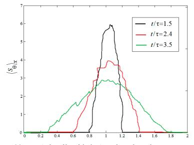
Figure 7. Mean vertical profiles of the horizontal rms thermal entropy generation.
