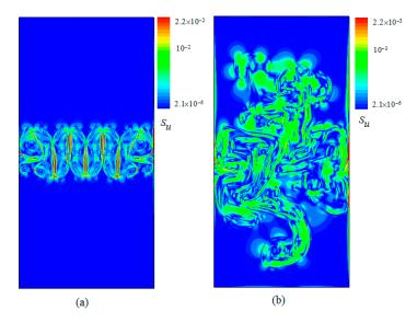
**Figure 4.** Snapshots of the viscous entropy generation with time evolution obtained at times (a)  $t/\tau = 1.2$ , and (b)  $t/\tau = 4$ .
