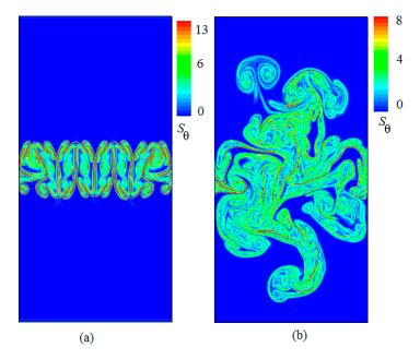
**Figure 5.** Snapshots of the thermal entropy generation with time evolution obtained at times (a)  $t/\tau = 1.2$ , and (b)  $t/\tau = 4$ .
