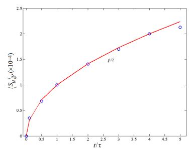
**Figure 8.** Temporal evolution of the viscous entropy generation rate normalized by the computational grid spacing.
