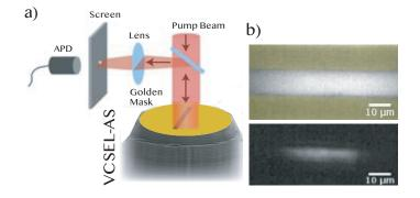
**Figure 1.** Experimental set up. (**a**) Schematic representation of an extended planar vertical cavity surface emitting laser with an integrated saturable absorber medium (VCSEL-SA). (**b**) Right panels account for the top-view camera snapshots of the one-dimensional line VCSEL-SA surface below (upper image, with the mask visible) and above laser threshold (lower image).
