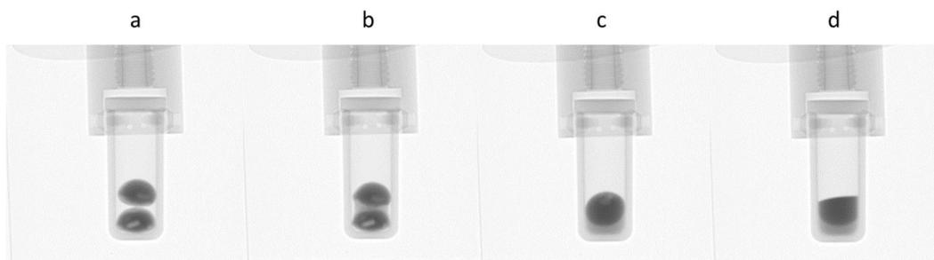
**Figure 8.** Melting and liquid phase separation of stacked CoCrCu samples. (a) During initial heating, the two as-cast buttons are intact; (b) the Cu-rich phase melts first between 1075 and 1100 °C and (c) pools at the bottom of the crucible; (d) the Cu-lean phase fully melts upon heating to 1500 °C and stacks based on density due to the influence of gravity. Images displayed with permission from the authors in [72].
