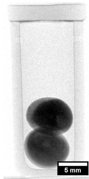
**Figure 9.** Neutron radiograph of two stacked arc-melted CoCrCu buttons in an alumina crucible with brighter regions corresponding to Cu-rich phases and darker regions corresponding to CoCr-rich phases. Image displayed with permission from the authors in [72].
