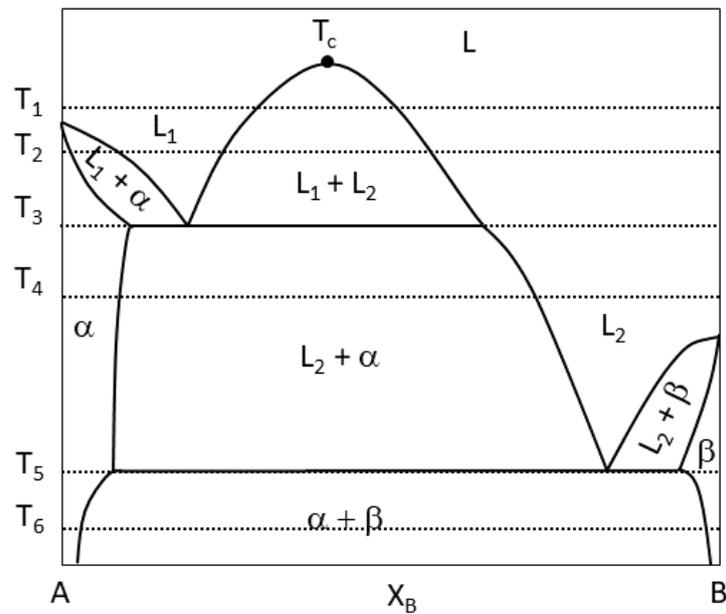
Figure 1. Generalized equilibrium monotectic binary phase diagram.
