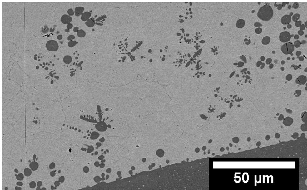
**Figure 7.** Backscattered electron image displaying emulsion and protrusions of the CoCr-rich (darker) phase into the Cu-rich (lighter) phase in an as-cast alloy of CoCrCu.
