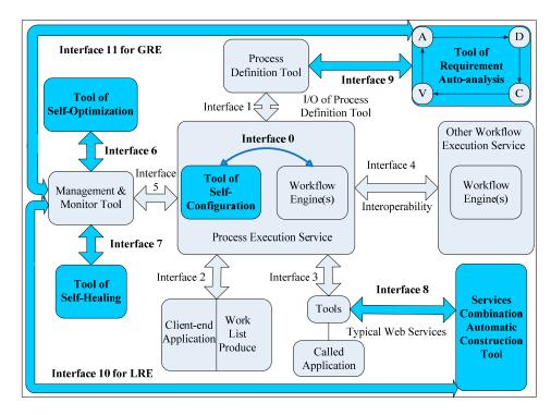
**Figure 1.** Reference model for a trustworthy workflow management system (TWfMS) with resilience engineering (RE).
