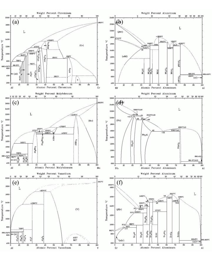
S1. Y-Al phase diagrams where Y is (a) Cr, (b) Hf, (c) Mo, (d) Nb, (e) V, and (f) Zr [18]. Nb and Zr were excluded due to relatively small solubility limit.
