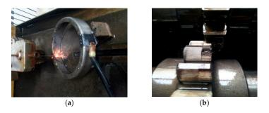
Figure 16. Bearing and gear fault diagram. (a) Bearing outer ring defect; (b) Gear peeling.
