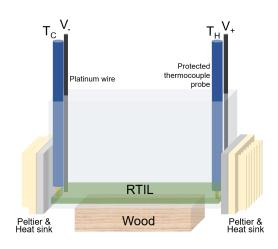
**Figure 2.** Experimental setup. The room-temperature ionic liquid (RTIL) fills only a few millimeters of the bottom of the quartz cuvette. The cold and hot temperatures  $T_C$  and  $T_H$  determine the polarity of the measured voltage. Peltier coolers and heat sinks are afixed with thermal paste.
