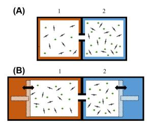
**Figure 5.** (**A**) Thermodynamic (N, V, T) isochoric model, where the volume of hot and cold cells (red and blue) are fixed; (**B**) Thermodynamic (N, P, T) isobaric model, where the cells have similar pressure but the volume of each cell is permitted to change.
