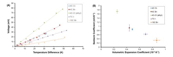
**Figure 4.** (A) Linearized changes in voltages as a function of temperature difference in order to estimate a linear Seebeck coefficient; (B) Negative correlation between volumetric heat expansion coefficient and linearized Seebeck coefficient. Error bars show variations in the linearized calculation of both coefficients.
