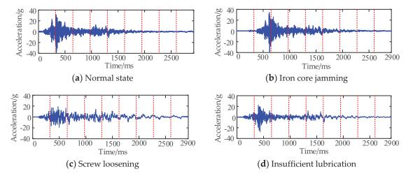
Figure 1. Time-domain division diagram of the original vibration signal.
