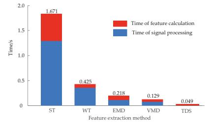
Figure 9. Feature extraction time of different methods.
