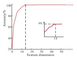
Figure 4. Accuracy of feature combination of different dimensions in forward feature selection.
