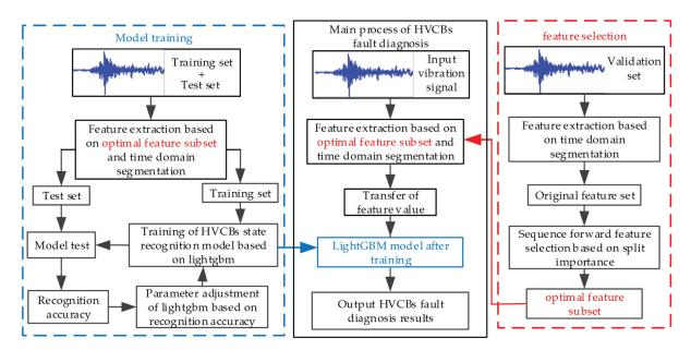
Figure 8. High voltage circuit breakers (HVCBs) fault diagnosis flow chart.
