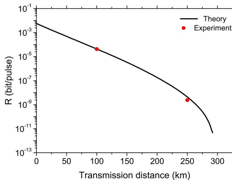
**Figure 4.** Theoretical and experimental results of the key rate's dependence on the transmission distance. system parameters are as follows: dark counting rate per pulse and overall efficiency of detection side are  $4 \times 10^{-8}$  and 60%; misalignment errors in Z and X bases are 0.15% and 1.5%, respectively.
