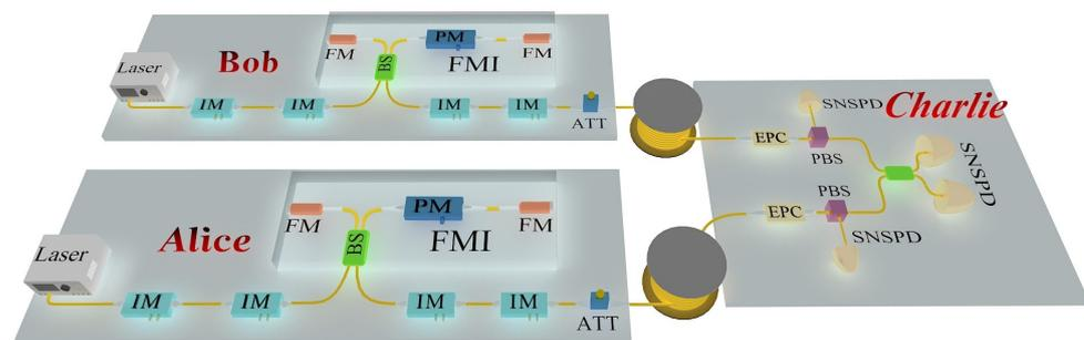
**Figure 3.** Schematic setup of MDI-QKD system. Laser, continuous-wave laser; IM, intensity modulator; PM, phase modulator; FM, Faraday mirror; ATT, attenuator; EPC, electronic polarization controller; BS: beam splitter; SNSPD, super-conducting nanowire single-photon detector.
