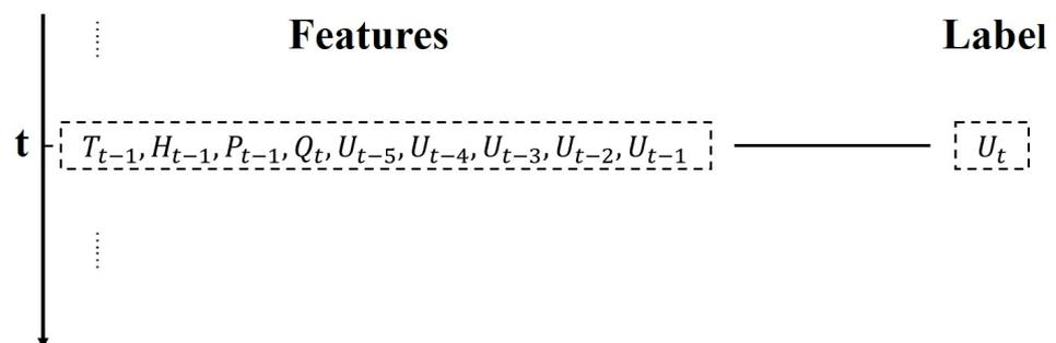
**Figure 1.** Data structure of  $t$  moment. T, temperature; H, humidity; P, intensity of laser; Q, QBER of  $XX$  basis-pair; U, voltage.
