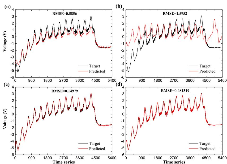
**Figure A1.** Comparisons of prediction results from (a) ARMA, (b) feed-forward neural network (one hidden layer with 50 neurons), (c) one-layer LSTM network, and (d) two-layer LSTM network.
