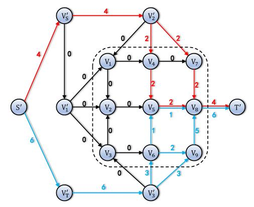
**Figure 7.** The max flow of auxiliary graph. The lines with same color represent the quantum key flow of same ground stations. The occupied traffic is drawn near the edges.
