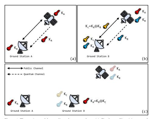
**Figure 1.** The storing and forwarding of quantum keys. (a): Firstly, satellite visits ground station A. Key  $K_A$  is generated between them by quantum link; (b): Secondly, satellite visits ground station B. Key  $K_B$  is generated between them by quantum link. Then, key  $K_C$  is generated by XOR operation of  $K_A$  and  $K_B$  by satellite and is sent by classical link. Ground station B decrypts  $K_C$  to obtain key  $K_A$ ; (c): Finally, ground stations A and B share same key  $K_A$ .
