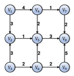
**Figure 5.** The network graph.  $V_8$  is the sink node. The edges always start from the nodes with greater hops and ends at smaller ones. The numbers of edges are the capacities of links.
