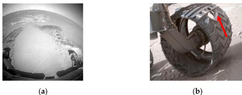
**Figure 1.** Risks to Mars rovers come from terrain: (a) Spirit rover sunk into the soil; (b) a puncture on a wheel of Curiosity.
