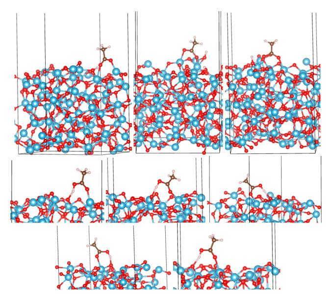
**Figure 5.** Adsorption configurations of AcOH on the "top" surface of a-TiO<sub>2</sub>. Top row: BB1 to BB3 (left to right). Bottom rows: M1 to M5 (left to right and top to bottom).
