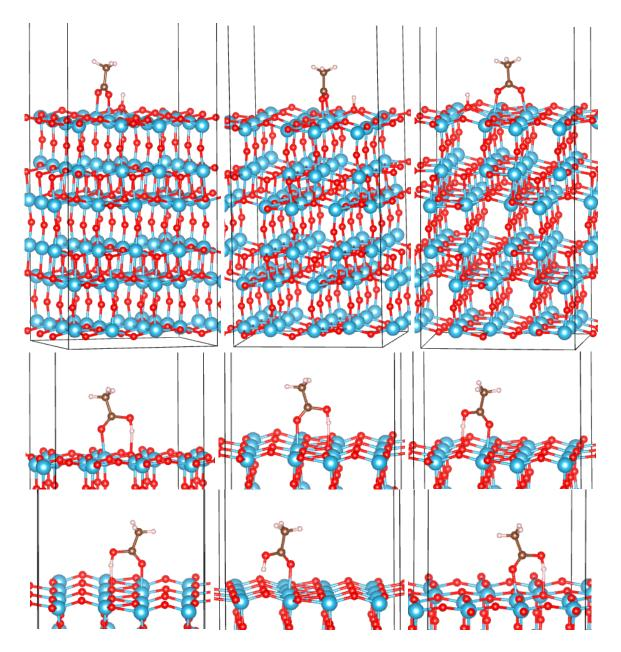
**Figure 4.** Adsorption configurations of AcOH on the (B) (001) surface of TiO<sub>2</sub>. Top row: BB1 to BB3 (left to right). Bottom rows: M1 to M6 (left to right and top to bottom).
