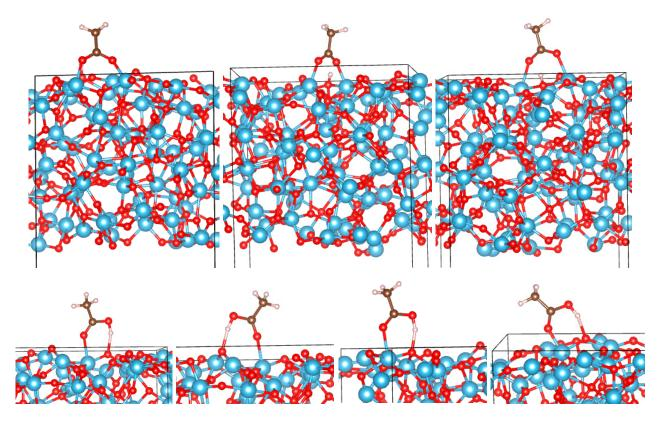
**Figure 6.** Adsorption configurations of AcOH on the "bottom" surface of *a*-TiO<sub>2</sub>. Top row: BB1 to BB3 (left to right). Bottom row: M1 to M4 (left to right).
