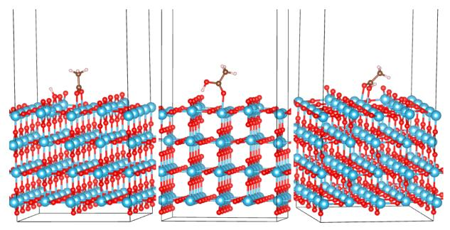
**Figure 3.** Adsorption configurations of AcOH on the rutile (110) surface of TiO<sub>2</sub>: BB (left), M1 (middle) and M2B (right).
