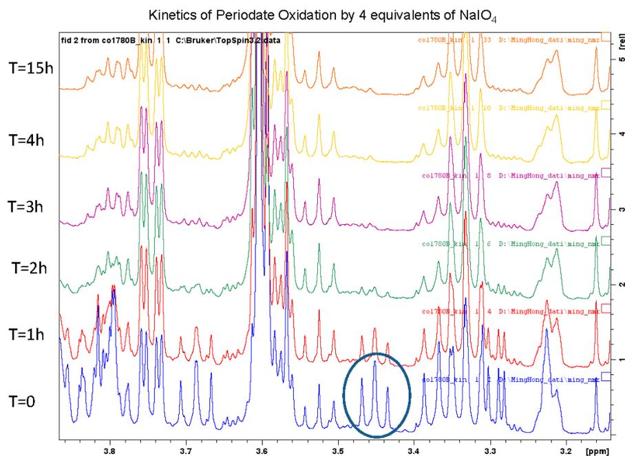
**Figure S1.**  $^1\text{H-NMR}$  spectra used to monitor the periodate oxidation of **1**. The circled signal that disappears throughout the reaction corresponds to H-2' of GlcA (3.44 ppm).
