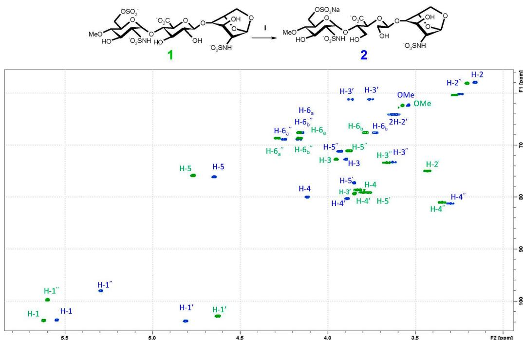
**Figure S3.** 2D HSQC spectra of compound **1** (green) and **2** (blue). (no quote, quote and double quote respectively refer to reducing-end unit, central unit and non reducing end unit).
