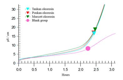
**Figure 3.** Oxidation curves obtained for the oleoresin samples extracted from the three citrus varieties as determined by Rancimat.
