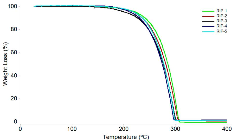
**Figure 4.** Dynamic thermogravimetric curves of riparin batches at the heating rate of 10.0 °C·min<sup>-1</sup>.
