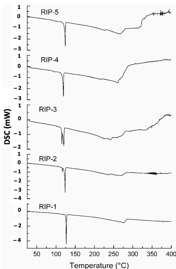
Figure 2. DSC curves of riparin I batches at the heating rate of  $2.0\text{ }^{\circ}\text{C}\cdot\text{min}^{-1}$ .
