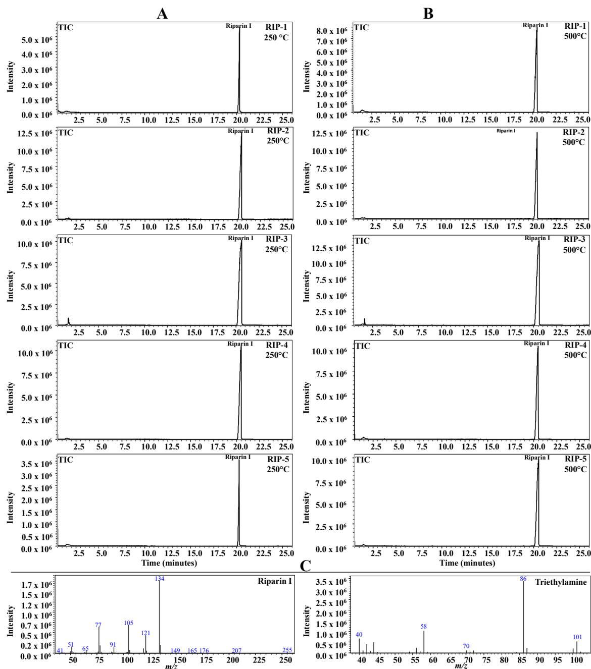
**Figure 6.** Pyrograms obtained from riparin at the temperatures of 250.0 °C (column (A)) and 500.0 °C (column (B)), showing the peak corresponding to riparin I and the product ion mass spectra of riparin I and triethylamine (column (C))—bottom of the figure).
