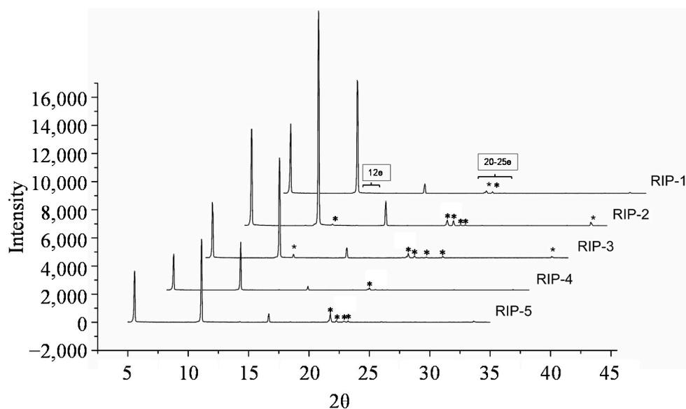
**Figure 7.** PXRD patterns of riparin I batches. The (\*) show characteristic diffraction pattern for each lot.
