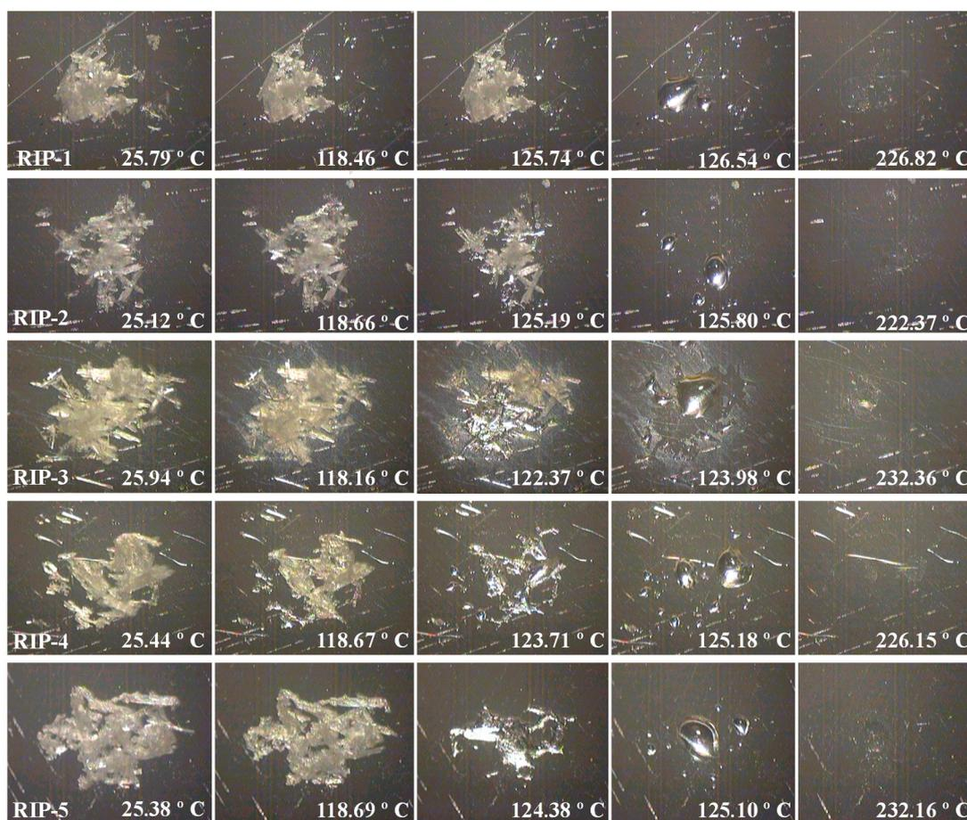
**Figure 3.** DSC-Photovisual of RIP-1, RIP-2, RIP-3, RIP-4, and RIP-5 samples in the heating 400 rate of 10 °C·min<sup>-1</sup>.
