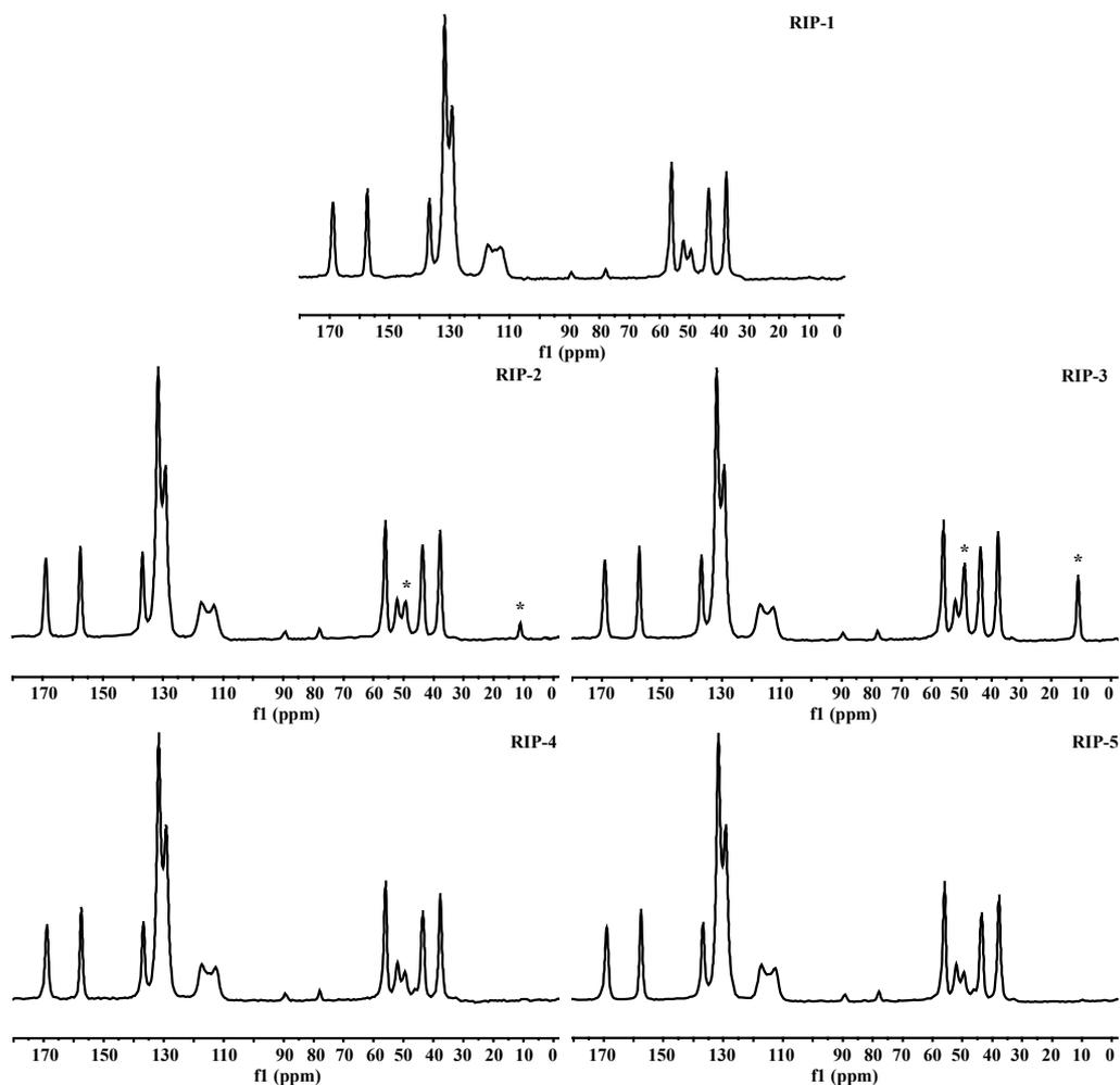
**Figure 8.** Solid-state  $^{13}\text{C}$ -NMR spectra of riparin I physical forms. The (\*) show characteristic peak corresponding of triethylamine.
