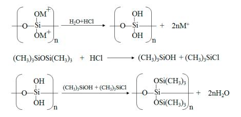
Scheme 3. Synthesis of MQ copolymers by trimethylsilylation of natural silicates.
