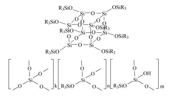
Figure 1. An ideal structure of a cubane M8Q8 and a real structure of MQ-copolymer.
