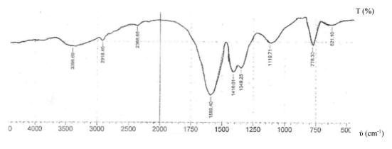
Figure 3. IR spectrum of [Nd(NBTCS)<sub>2</sub>(H<sub>2</sub>O)<sub>2</sub>]NO<sub>3</sub>.
