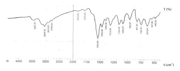
Figure 2. IR spectrum of N-(Benzothiazol-2-yl)-4-chlorobenzenesulphonamide (NBTCS).
