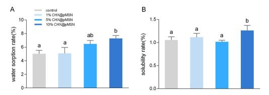
**Figure 7.** Water sorption rate (**A**) and solubility rate (**B**) of control, 1%, 5%, and 10% CHX@pMSN groups. Data are shown as mean  $\pm$  standard deviation. The groups labeled with the same letters have no significant difference (p > 0.05).
