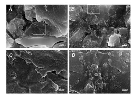
**Figure A1.** FESEM images of fracture surfaces from (**A**) 1% CHX@pMSN; and (**B**) 5% CHX@pMSN groups. (**C**,**D**) are magnified pictures of rectangles in (**A**,**B**) respectively. The nanoparticles dispersed uniformly in the GIC matrix and formed small agglomeration in 1% CHX@pMSN group. The agglomeration became larger in 5% CHX@pMSN group, however the dispersion of nanoparticles was uniform.
