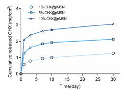
**Figure 8.** Release profile of cumulative CHX of 1%, 5%, and 10% CHX@pMSN groups at time points of 1, 3, 7, 10, and 30 days. All specimens were stored in distilled water at 37 °C.
