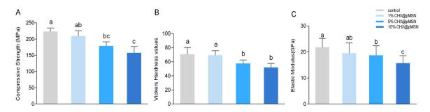
**Figure 5.** Mechanical properties of control, 1%, 5%, and 10% CHX@pMSN groups. (**A**) Compressive strength; (**B**) Vickers hardness; and (**C**) elastic modulus. Data are shown as mean  $\pm$  standard deviation. The groups labeled with the same letters have no significant difference (*p* > 0.05).
