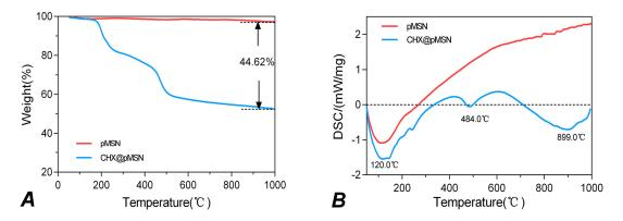
**Figure 2.** The thermogravimetric analysis for pMSN and CHX@pMSN shows (**A**) TGA curves; and (**B**) DSC curves.
