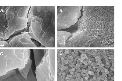
**Figure 6.** FESEM images of fracture surfaces from (**A**) control; and (**B**) 10% CHX@pMSN groups. (**C**,**D**) are magnified pictures of rectangles in (**A**,**B**) respectively.
