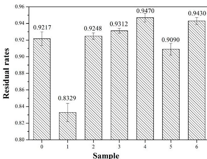
**Figure 2.** Residual rates of different adhesive samples: 0 (12 wt% soy protein isolate (SPI)), 1 (18 wt% SPI/bromelain), 2 (18 wt% SPI/bromelain/3 wt% TGA), 3 (18 wt% SPI/bromelain/6 wt% TGA), 4 (18 wt% SPI/bromelain/9 wt% TGA), 5 (18 wt% SPI/bromelain/12 wt% TGA), and 6 (18 wt% SPI/9 wt% TGA).
