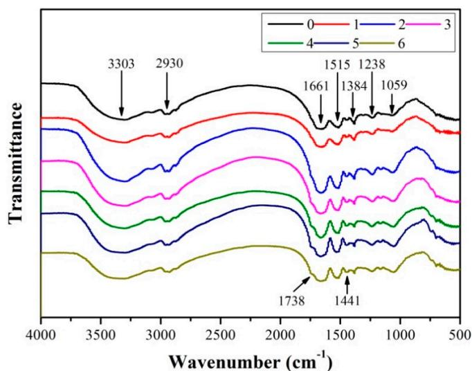
**Figure 5.** Fourier-transform infrared spectra of the different adhesive samples: 0 (12 wt% SPI), 1 (18 wt% SPI/bromelain), 2 (18 wt% SPI/bromelain/3 wt% TGA), 3 (18 wt% SPI/bromelain/6 wt% TGA), 4 (18 wt% SPI/bromelain/9 wt% TGA), 5 (18 wt% SPI/ bromelain/12 wt% TGA), and 6 (18 wt% SPI/ 9 wt% TGA).
