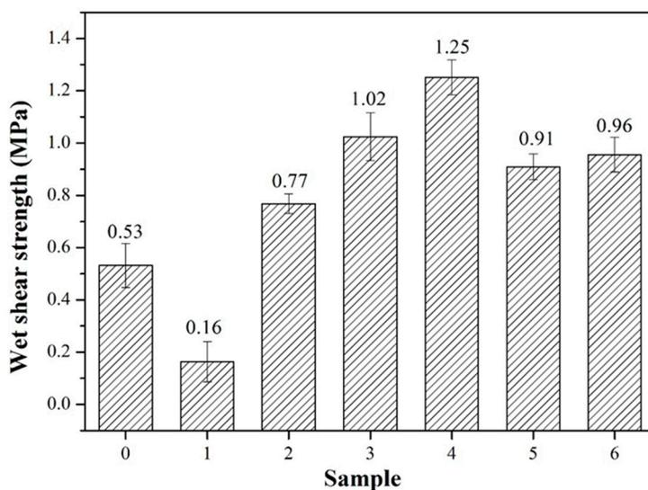
**Figure 3.** Wet shear strength of the different adhesive samples: 0 (12 wt% SPI), 1 (18 wt% SPI/bromelain), 2 (18 wt% SPI/bromelain/3 wt% TGA), 3 (18 wt% SPI/bromelain/6 wt% TGA), 4 (18 wt% SPI/bromelain/9 wt% TGA), 5 (18 wt% SPI/bromelain/12 wt% TGA), and 6 (18 wt% SPI/9 wt% TGA).
