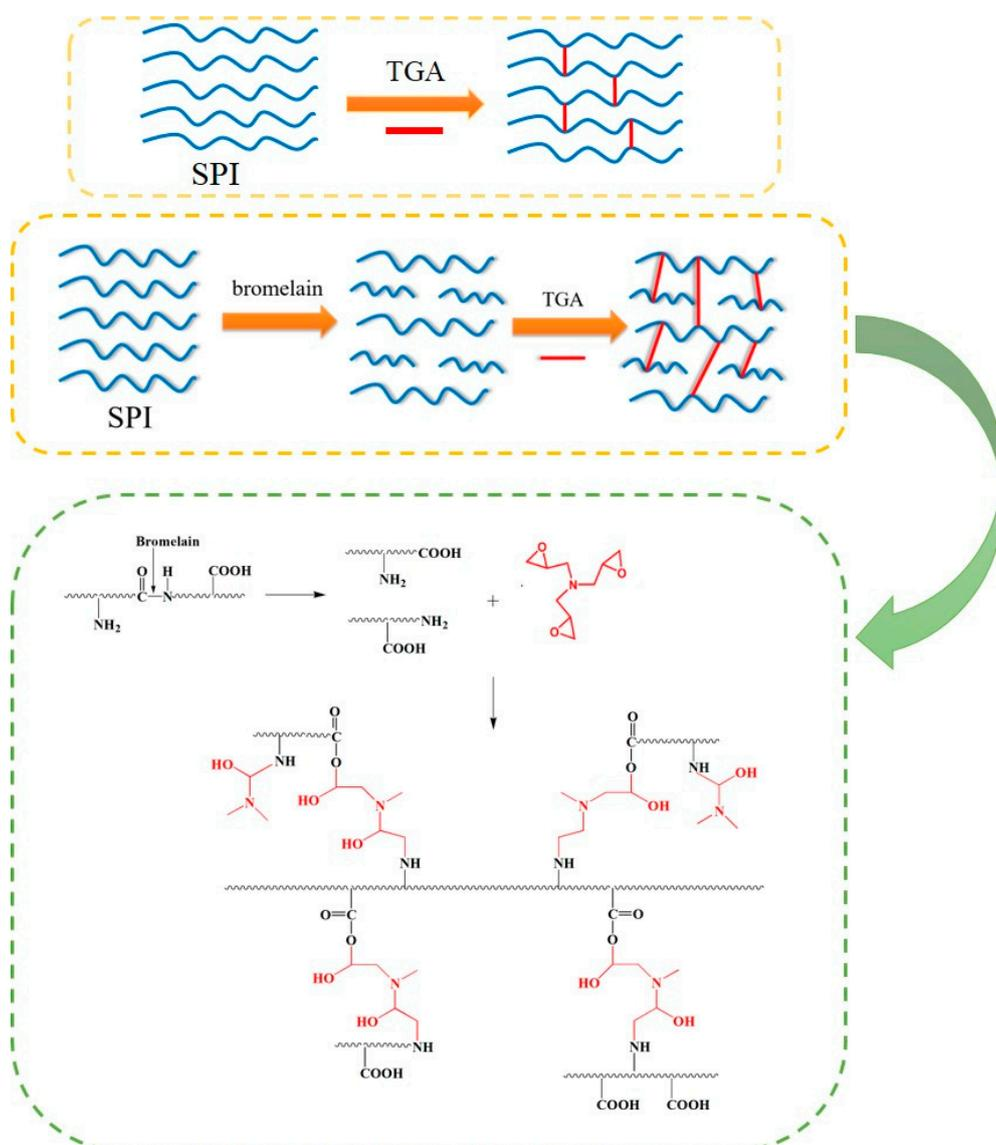
**Figure 4.** Cross-linking network of the soy protein adhesive.
