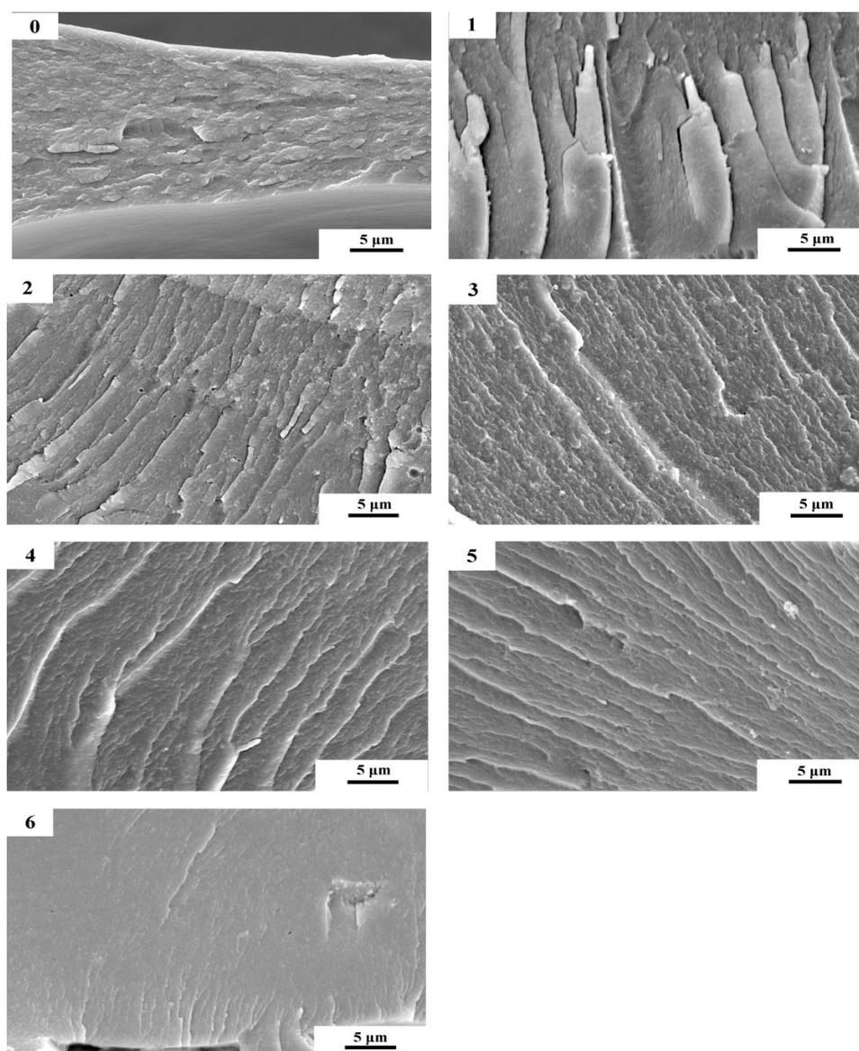
**Figure 7.** Fracture surface micrographs of the different cured adhesive samples: 0 (12 wt% SPI), 1 (18 wt% SPI/bromelain), 2 (18 wt% SPI/bromelain/3 wt% TGA), 3 (18 wt% SPI/bromelain/6 wt% TGA), 4 (18 wt% SPI/bromelain/9 wt% TGA), 5 (18 wt% SPI/bromelain/12 wt% TGA), and 6 (18 wt% SPI/9 wt% TGA).
