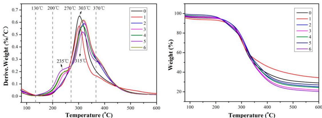
**Figure 6.** Thermogravimetric (TG, left) and derivative thermogravimetric (DTG, right) curves of the different adhesive samples: 0 (12 wt% SPI), 1 (18 wt% SPI/bromelain), 2 (18 wt% SPI/bromelain/3 wt% TGA), 3 (18 wt% SPI/bromelain/6 wt% TGA), 4 (18 wt% SPI/bromelain/9 wt% TGA), 5 (18 wt% SPI/bromelain/12 wt% TGA), and 6 (18 wt% SPI/9 wt% TGA).
