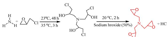
**Figure 1.** The synthesis procedure of cross-linker triglycidylamine (TGA).
