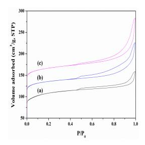
**Figure 2.** Adsorption/desorption isotherms of nitrogen at 77 K on the alkaline-treated ZSM-5 and the parent ZSM-5 zeolites: (a) H-Z-0; (b) H-Z-20; and (c) H-Z-30. For clarity the isotherms of H-Z-20 and H-Z-30 have been shifted upward by 50 cm<sup>3</sup>/g and 100 cm<sup>3</sup>/g, respectively.
