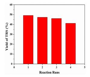
**Figure 9.** Yield of TRS vs. catalytic cycles of H-Z-30 in hydrolysis of cellulose. Reaction conditions: [BMIm]Cl (1.0 g), cellulose (50.0 mg), catalyst (50.0 mg), water (0.2 mL), at 403 K and 2 h.
