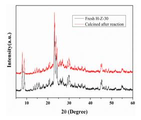
Figure 8. XRD patterns of fresh H-Z-30 and calcined H-Z-30 after the cellulose hydrolysis.
