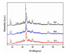
**Figure 1.** XRD patterns of the alkaline-treated ZSM-5 and the parent ZSM-5 zeolites: (**a**) H-Z-0; (**b**) H-Z-20; and (**c**) H-Z-30.
