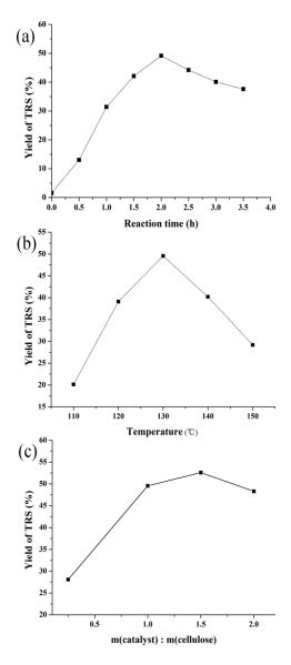
**Figure 5.** The effect of reaction time (**a**); temperature (**b**); and weight ratio of catalysts to cellulose (**c**) on TRS yields over H-Z-30. Reaction conditions: [BMIm]Cl (1.0 g), water (0.2 mL).
