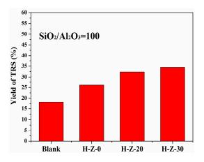
**Figure 4.** Hydrolysis of cellulose catalyzed by the alkaline-treated ZSM-5 and the parent ZSM-5 zeolites with  $SiO_2/Al_2O_3$  ratio of 100. Reaction conditions: [BMIm]Cl (1.0 g), cellulose (50.0 mg), catalyst (50.0 mg), water (0.2 mL), at 403 K and 2 h.
