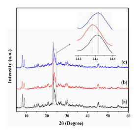
**Figure 6.** XRD patterns of H-Z-30 before and after IL-treatments. (**a**) H-Z-30; (**b**) IL-treated H-Z-30; and (**c**) samples of calcined IL-treated H-Z-30 at 823 K for 5 h.
