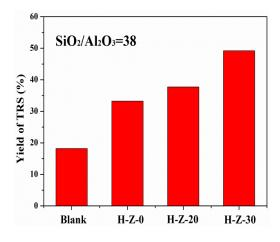
**Figure 3.** Hydrolysis of cellulose catalyzed by the alkaline-treated ZSM-5 and the parent ZSM-5 zeolites with  $SiO_2/Al_2O_3$  ratio of 38. Reaction conditions: [BMIm]Cl (1.0 g), cellulose (50.0 mg), catalyst (50.0 mg), water (0.2 mL), at 403 K and 2 h.
