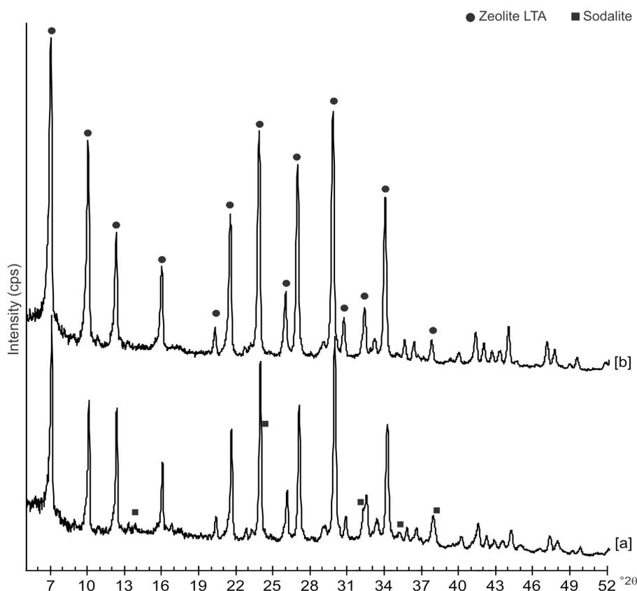
**Figure 1.** XRD patterns of samples synthesized after 4 day of: [a] hydrothermal process with ultrasonic irradiation and [b] conventional hydrothermal treatment.
