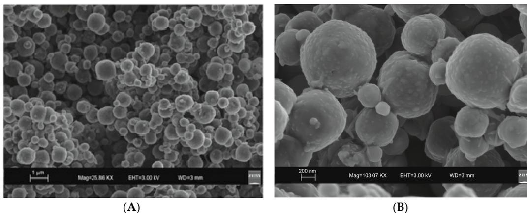
**Figure 4.** SEM images of LTA zeolite formed by a 4-day conventional hydrothermal incubation. (A) overview of zeolites formed; (B) zoom in on LTA crystals.
