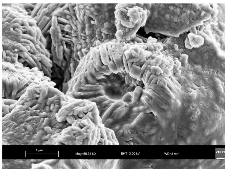
**Figure 7.** SEM image showing well defined plate morphology of sodalite crystal formed 6 months after hydrothermal treatment with ultrasonic.
