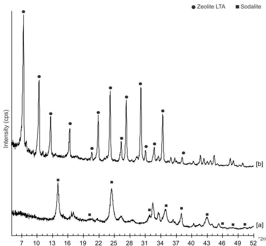
**Figure 2.** XRD profiles of sample analyzed: [a] 6 months after the synthesis by hydrothermal process with ultrasonic irradiation and [b] 12 months after the synthesis by conventional hydrothermal treatment.
