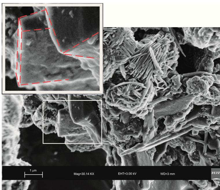
**Figure 8.** SEM image showing cubic face morphology of relict LTA zeolite (highlighted and enlarged part) detectable between sodalite crystals.
