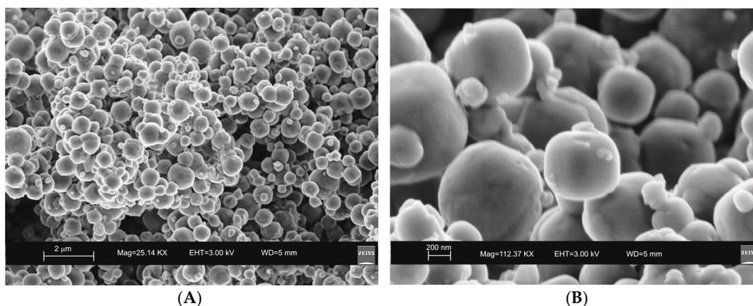
**Figure 6.** SEM images of LTA zeolite characterizing the sample 12 months after the conventional hydrothermal treatment. (A) overview of zeolites formed; (B) zoom in on LTA crystals.
