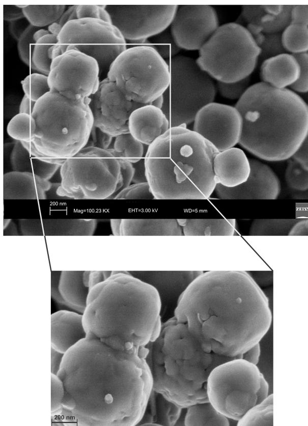
**Figure 9.** SEM images of sample 12 months after the synthesis by HY. They show isolated LTA crystal affected by an initial process of transformation into sodalite.
