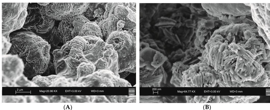
**Figure 5.** SEM images of sodalite characterizing the sample 6 months after the ultrasonic water bath treatment. (A) overview of zeolites formed; (B) detail of sodalite crystal.
