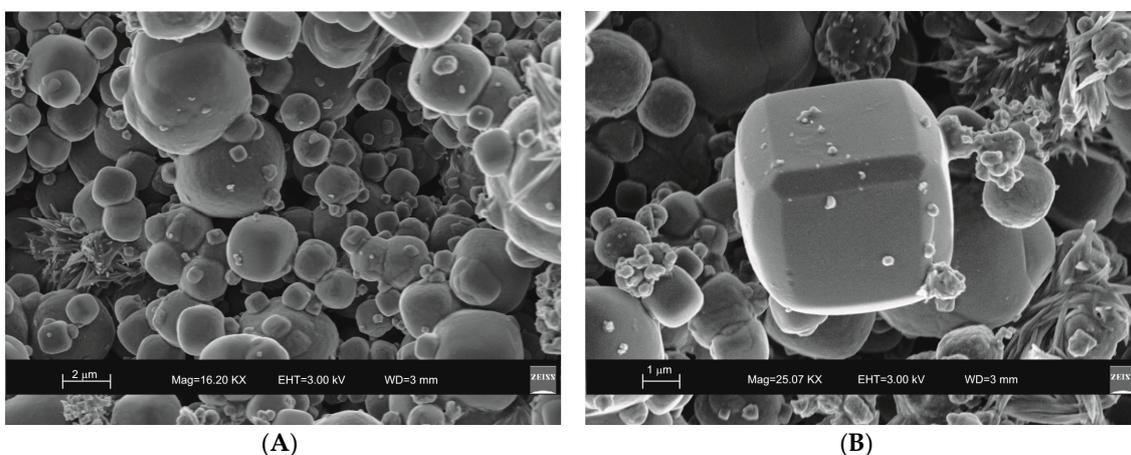
**Figure 3.** Scanning electron microscopy (SEM) images of LTA zeolite formed through 45 min of hydrothermal process with sonication. (A) overview of zeolites formed; (B) detail of LTA crystal.
