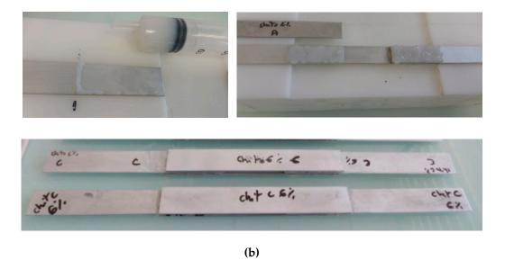
**Figure 4.** Illustration of bonded double-lap wood (**a**) and aluminium (**b**) specimens prepared for the mechanical characterization.
