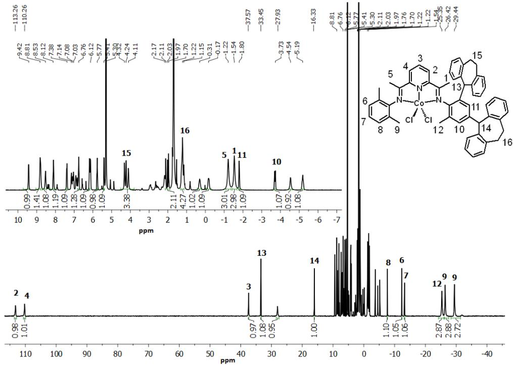
Figure S1  $^1\text{H}$  NMR spectrum of **Co1** in  $\text{CD}_2\text{Cl}_2$  at room temperature.
