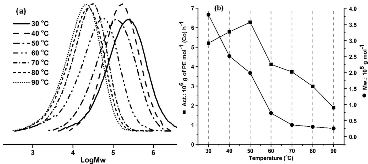
**Figure S6** GPC curves of the obtained polyethylene **(a)**; activity and  $M_w$  as a function of reaction temperature **(b)** for the **Co1**/MMAO system (Table 5, entries 1 – 7).
