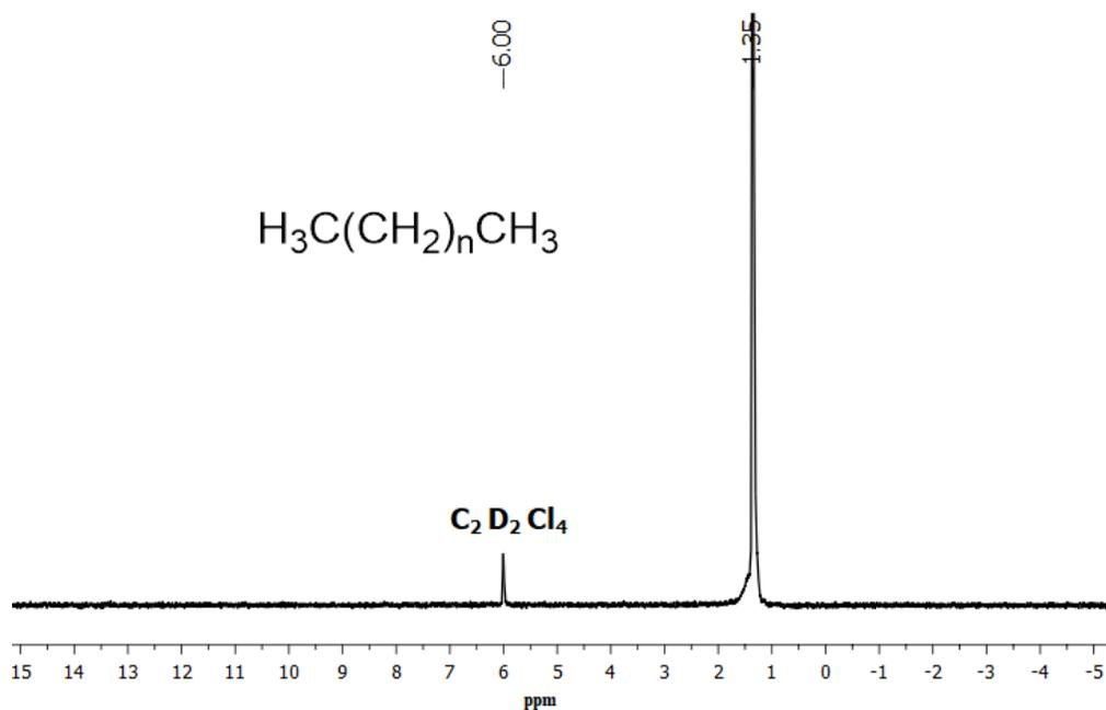
**Figure S11** The  $^1\text{H}$  NMR spectrum of the polyethylene obtained with **Co1**/MMAO (Table 5, entry 10).
