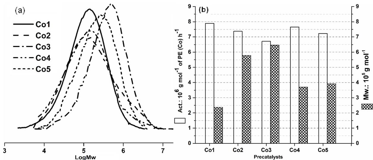
**Figure S9** GPC curves of the obtained polyethylene (a); activity and  $M_w$  for different precatalysts (b) at the optimized reaction conditions with MMAO as cocatalyst (Table 6, entries 1 – 5).
