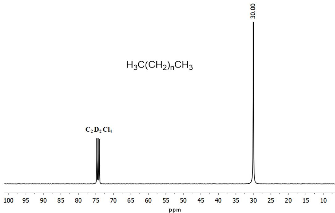
**Figure S12** The  $^{13}\text{C}$  NMR spectrum of the polyethylene obtained with **Co1**/MMAO (Table 5, entry 10).
