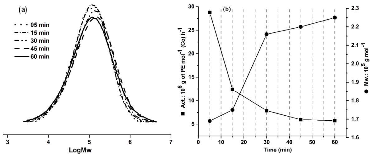
**Figure S8** GPC curves of the obtained polyethylene (a); activity and  $M_w$  as a function of run time (b) for the Co1/MMAO system (Table 5, entries 10 and 14 – 17).
