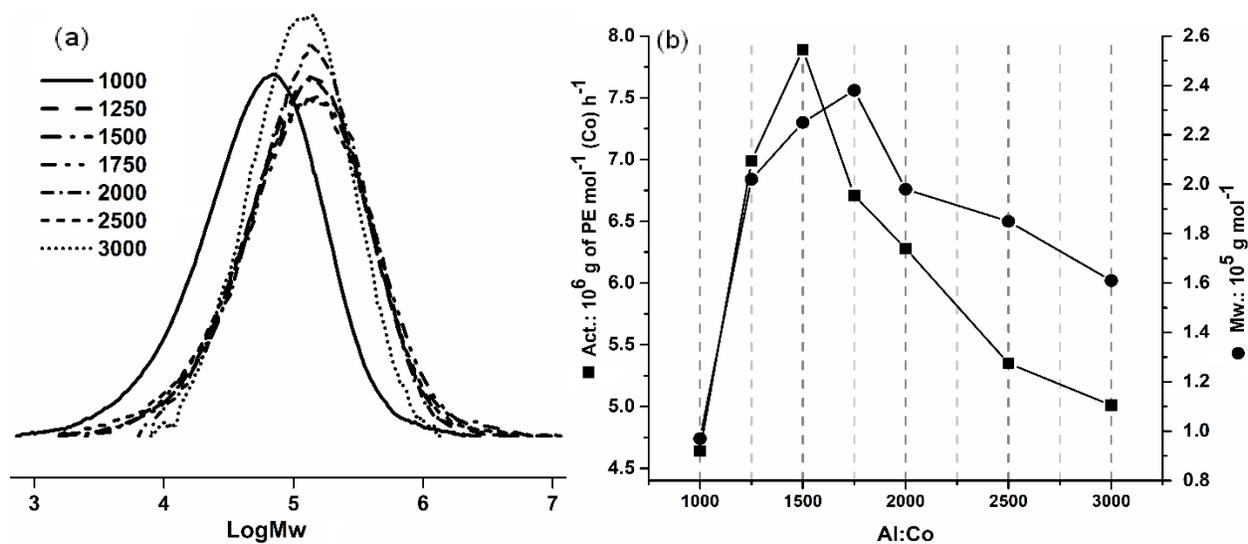
**Figure S7** GPC curves of the obtained polyethylene (a); activity and  $M_w$  as a function of Al/Co ratio (b) for the Co1/MMAO system (Table 5, entries 3 and 8 – 13).
