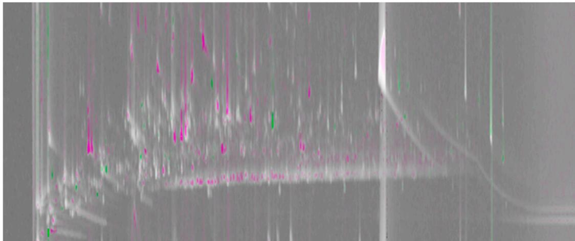
**Figure 1.** A comparative visualization between composite GC×GC/MS chromatograms of the high (reference image) and low (analyzed image) elevation teas. The magenta and green peak regions show the areas in the chromatogram where relative distribution of common analytes is higher in the high and low elevation teas, respectively. Light grey peak regions correspond to analytes with similar percentage response in the two chromatograms.
