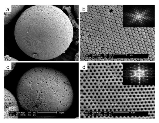
**Figure 3.** (**a**,**b**) SEM images of spherical opal composite structures consisting of PS/HEMA nanoparticles and titania nanoparticles. (**c**,**d**) SEM images of spherical titania inverse opal structure. Inset shows the fast Fourier transform (FTT) of the SEM images.
