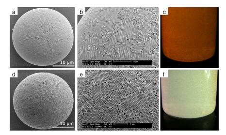
**Figure 2.** (**a**,**b**) SEM images and (**c**) digital camera image of spherical opal structures made of 280 nm-sized PS/HEMA nanoparticles. (**d**,**e**) SEM images and (**f**) digital camera image of spherical opal structures from 210-nm-sized PS/HEMA nanoparticles.
