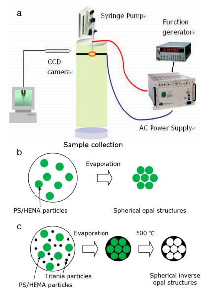
**Scheme 1.** (a) Schematic of experimental set up of electro-hydrodynamic atomization for generating uniform droplets. Schematics of self-assembly processes of (b) spherical PS/HEMA opal structures and (c) spherical titania inverse opal structures.
