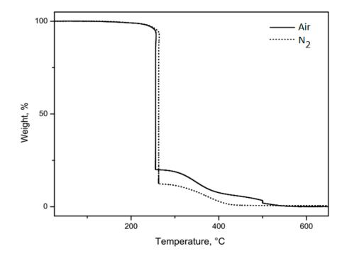
**Figure 3.** TG/DTG curve: Mass loss of babassu oil in an oxidative atmosphere of synthetic air and nitrogen under almost quasi-isothermal conditions.
