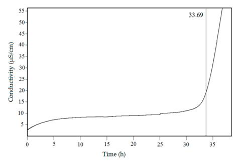
**Figure 1.** Conductivity versus time determined by the Rancimat method. Oxidation stability of oils at 110 °C. The induction time of babassu oil was 33.69 h.
