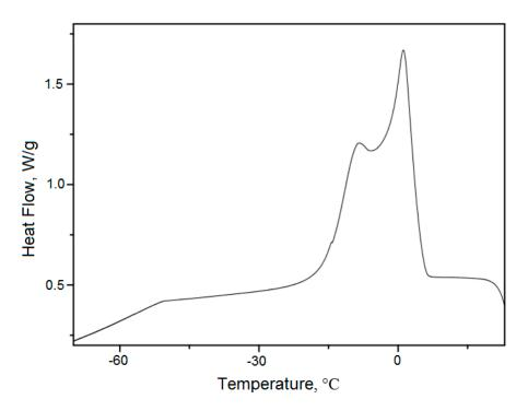
**Figure 4.** Cooling of babassu oil on an oxidative atmosphere of nitrogen under almost quasi-isothermal conditions.
