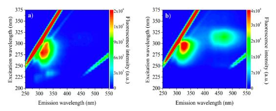
**Figure 6.** Excitation-emission map of oils from the babassu obtained by exciting between 200–375 nm and emission in the 250–550 nm range (concentration: (**a**)  $1 \times 10^{-3}$  and (**b**) 0.05 g/mL).
