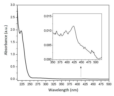
**Figure 5.** UV-VIS absorption spectrum (wavelength from 210 to 500 nm) of babassu oil diluted in hexane at 0.0100 g  $L^{-1}$ ). Inset: Zoom of the UV-Vis spectrum in the 350 to 500 nm range.
