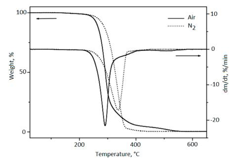
**Figure 2.** TG/DTG curve: Mass loss of babassu oil in an oxidative atmosphere of synthetic air and nitrogen under dynamic condition.
