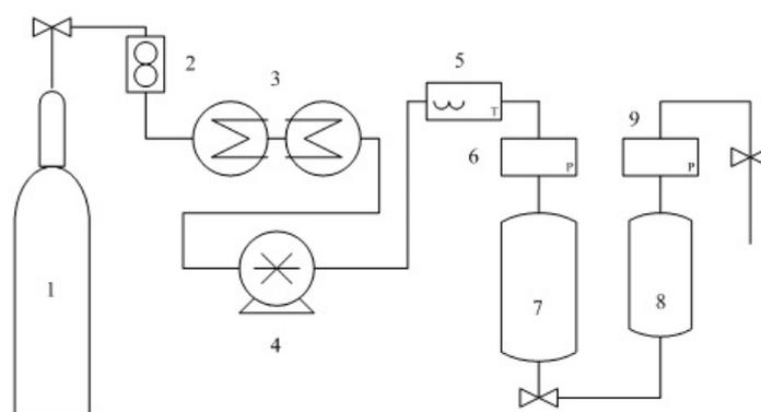
**Figure 3.** Scheme of the experimental set-up for supercritical CO<sub>2</sub> fluid extraction. 1: CO<sub>2</sub> feed tank; 2: flow meter; 3: cryostat; 4: pump; 5: heater; 6: manometer; 7: extraction tank; 8: Separation tank; 9. manometer.
