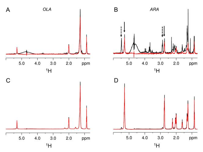
**Figure S1**. *Translational diffusion of fatty acids*. The displayed NMR diffusion spectra were recorded with 5% (black) and 95% (red) of the maximum gradient strength (53.5 G/cm) and a diffusion delay of 200 ms. The samples contained 75  $\mu$ M OLA (A), 75  $\mu$ M ARA (B), 500  $\mu$ M OLA (C), or 500  $\mu$ M ARA (D). Peaks indicated by dashed (solid) arrows are assigned to ARA monomers (micelles). The measurement temperature was 37 °C.
