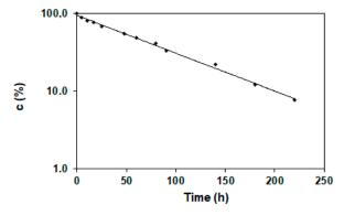
**Figure 7.** Semilogarithmic plot of the degradation of CIL@LC-2a (1:1 wt./wt.) product at 90 °C and humidity 76.4%.
