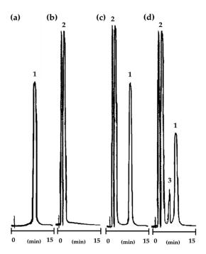
**Figure 6.** RP-HPLC chromatograms for: cilazapril in pure (a), LC-2a (1:1 wt./wt.) (b), CIL@LC-2a (1:1 wt./wt.) before degradation (c) and CIL@LC-2a (1:1 wt./wt.) after degradation (d). Retention times: cilazapril (1):  $t_R \sim 8$  min; LC-2a (1:1 wt./wt.) (2):  $t_R \sim 2-4$  min and degradation product of cilazapril (3):  $t_R \sim 6$  min.
