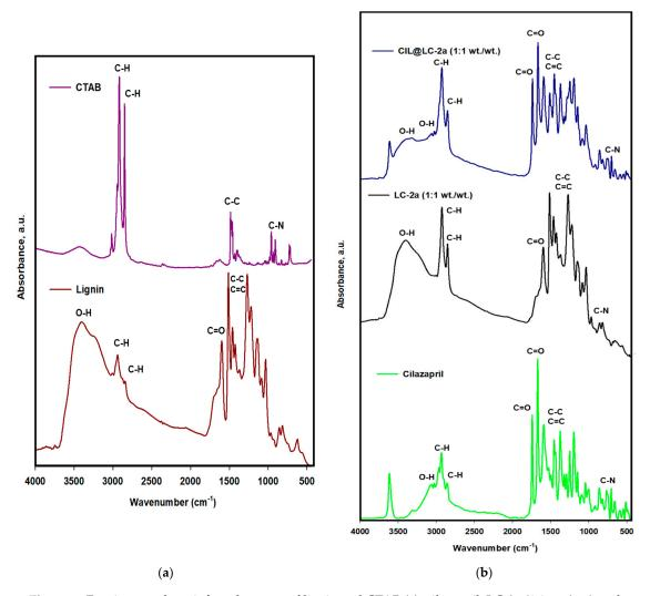
**Figure 3.** Fourier transform infrared spectra of lignin and CTAB (a), cilazapril, LC-2a (1:1 wt./wt.) and CIL@LC-2a (1:1 wt./wt.) (b).
