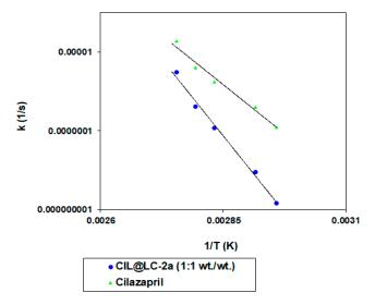
**Figure 8.** Semilogarithmic linear dependence of the reaction rate constant and the inverse of temperature for stability evaluation of cilazapril in pure and CIL@LC-2a (1:1 wt./wt.).
