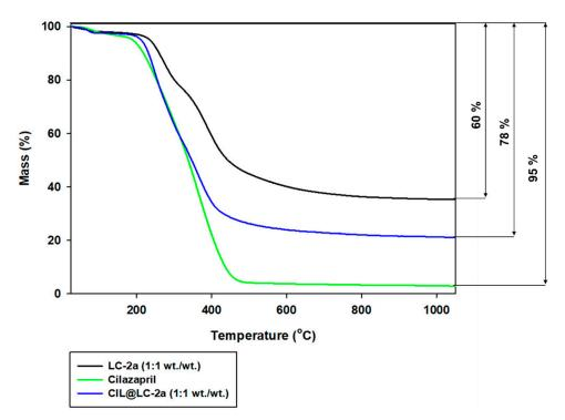
Figure 5. TGA curves of LC-2a (1:1 wt./wt.), cilazapril and CIL@LC-2a (1:1 wt./wt.).
