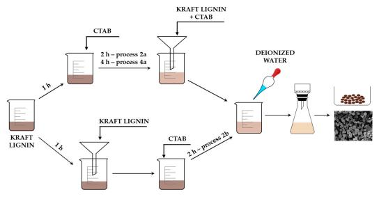
Figure 9. Schematic diagram of preparation of lignin-based spherical particles.
