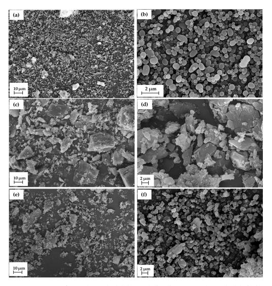
**Figure 2.** SEM images of LC-2a (1:1 wt./wt.) (**a,b**), CIL (**c,d**) and CIL@LC-2a (1:1 wt./wt.) (**e,f**); shown in two magnifications.
