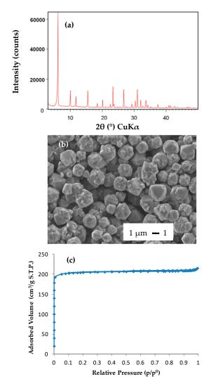
**Figure 1.** Pure 13X zeolite powder (FAU): (**a**) X-ray diffraction (XRD) pattern; (**b**) scanning electron micrograph; (**c**) nitrogen adsorption-desorption isotherms at –196 °C.
