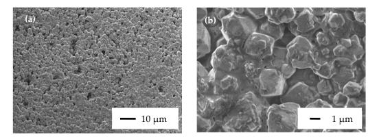
**Figure 3.** SEM micrographs of the zeolite FAU-HK46 coating 4 made with a zeolite content of 80 wt.% at different scales (**a**) 10  $\mu$ m; (**b**) 1  $\mu$ m.
