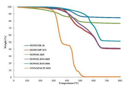
**Figure 2.** TGA (Thermogravimetric analyses) curves of commercial polymerized binders showing the weight loss as a function of the temperature (°C).
