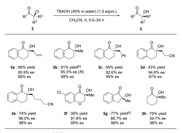
**Figure 2.** Substrate scope <sup>[a]</sup> (<sup>[a]</sup> Reactions were carried out with 1.5 equiv. of TBAOH at ambient temperature in acetnitrile, unless otherwise noted. <sup>[b]</sup> Reaction was carried out at 0 °C. <sup>[c]</sup> Reaction was carried out with 3.0 equiv. of TBAOH at 0 °C. es: enantiospecificity).
