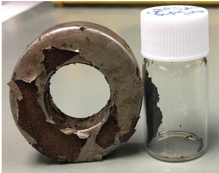
**Figure S11:** Photograph of MNPs being extracted by an external magnet.
