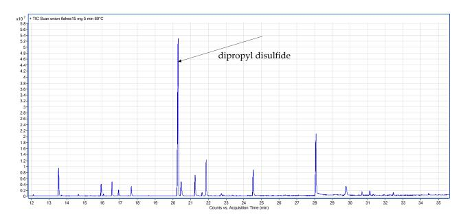
**Figure S2.** TIC of 15 mg onion flakes sample adsorbed for 5 min at  $60^{\circ}$ C.
