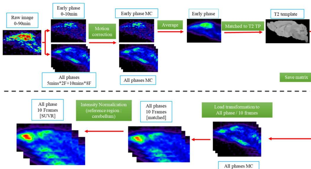
**Figure 2.** The procedure for creating the PET imaging template for each animal for further PET image analysis applied a rigid match with the MNI MRI T2 template.
