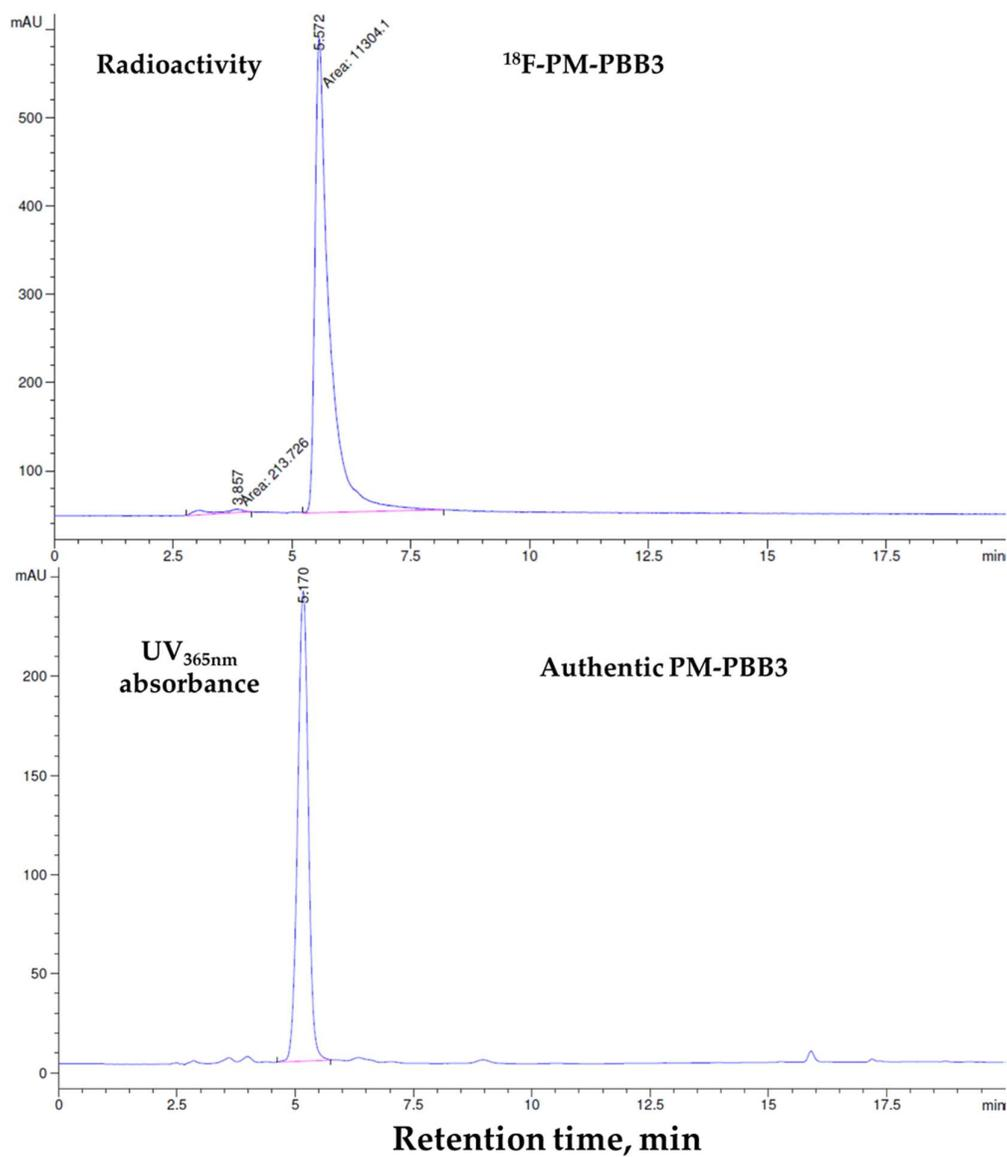
**Figure 1.** HPLC Profile of  $^{18}\text{F}$ -PM-PBB3.
