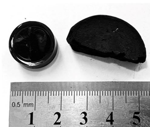
**Figure 2.** (Left) A non-porous dry organic xerogel upon collapse of nanoporosity (significant drying shrinkage) and (right) corresponding macroporous xerogel (obtained with the addition of isopropanol as an antisolvent), which did not undergo collapse of porosity and shrinkage during drying.
