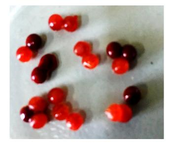
Figure 1. Microscopy image of alginate microcapsules loaded with capsaicin.
