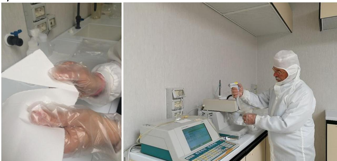
**Figure S8.** (a) Filter conditioning and weighing in the clean laboratory of Concordia Station, Antarctica. (b) Filter cutting and voltammetric analysis in our clean chemistry laboratory, Italy.
