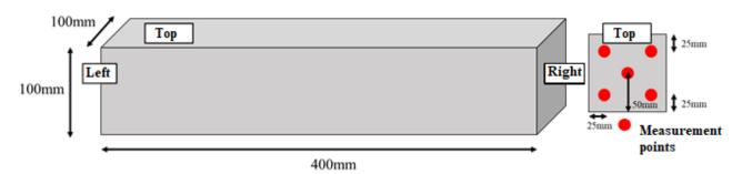
Figure 15. Measurements of cement mortar specimens.
