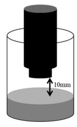
Figure 14. Spectral measurement immediately after mixing (cement paste).
