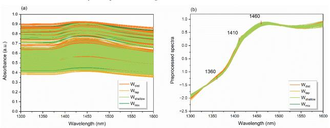
**Figure 4.** Near infrared spectra of cement paste and mortar samples created using different waters: (a) Raw absorbance spectra; (b) Preprocessed spectra using linear detrend correction and standard normal variate transformation.
