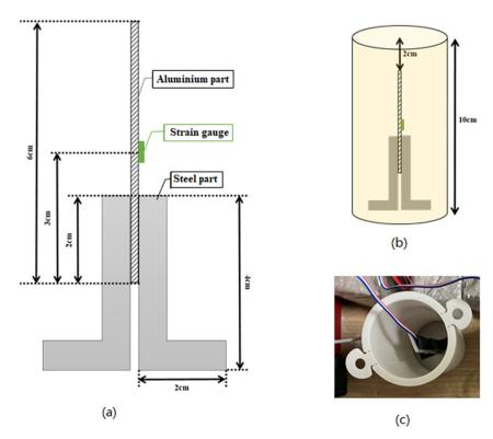
**Figure 16.** Measurements of the thermal changes of the cement paste; the method of fixing the strain gauge: (a) schematic representation of attached strain gauge, (b) arrangement of the jig in the formwork, and (c) experimental setup.
