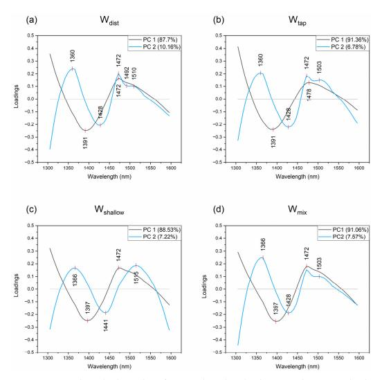
**Figure 6.** PC1 and PC2 loadings plots of PCA analysis describe changes in the water molecular structure during hardening of cement mortar prepared with different mixing water: (a)  $W_{tap}$ , (b)  $W_{mix}$ , (c)  $W_{dist}$ , and (d)  $W_{shallow}$ .
