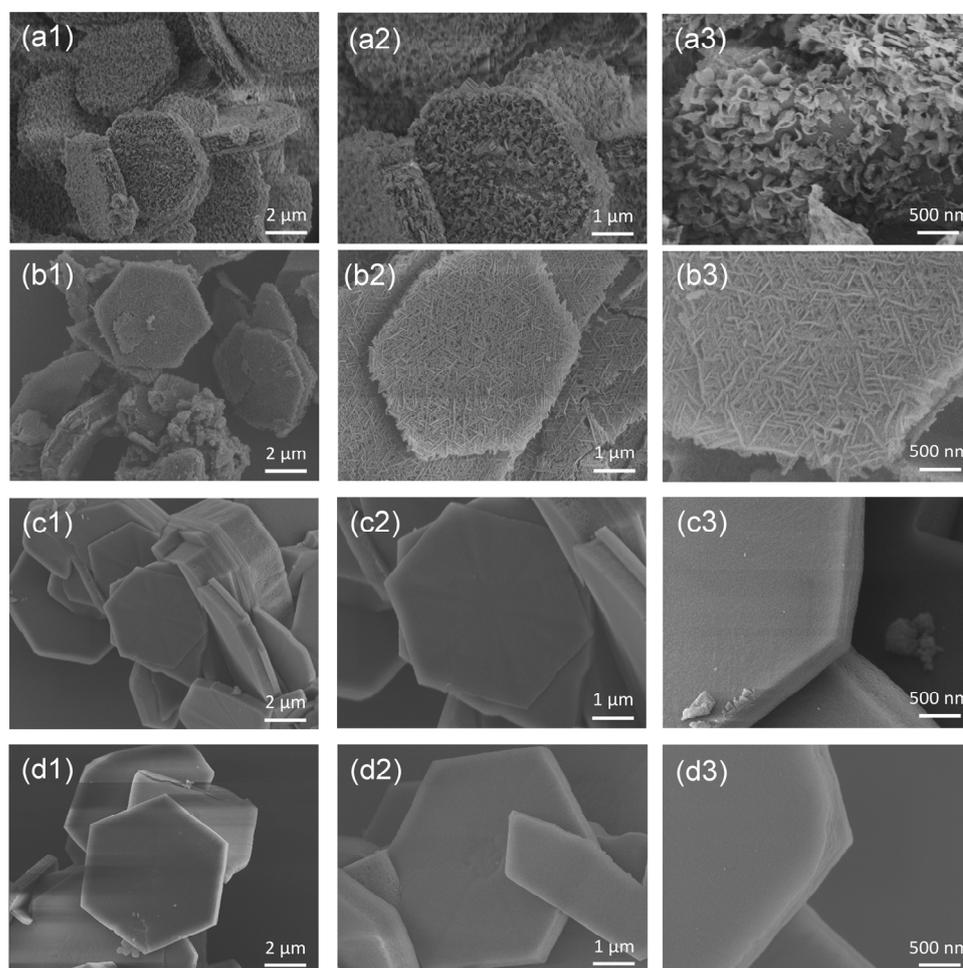
**Figure 1.** SEM images of Ni-MOF produced at different reaction temperatures, (a1–a3) Ni-MOF-60; (b1–b3) Ni-MOF-80; (c1–c3) Ni-MOF-100, and (d1–d3) Ni-MOF-120.
