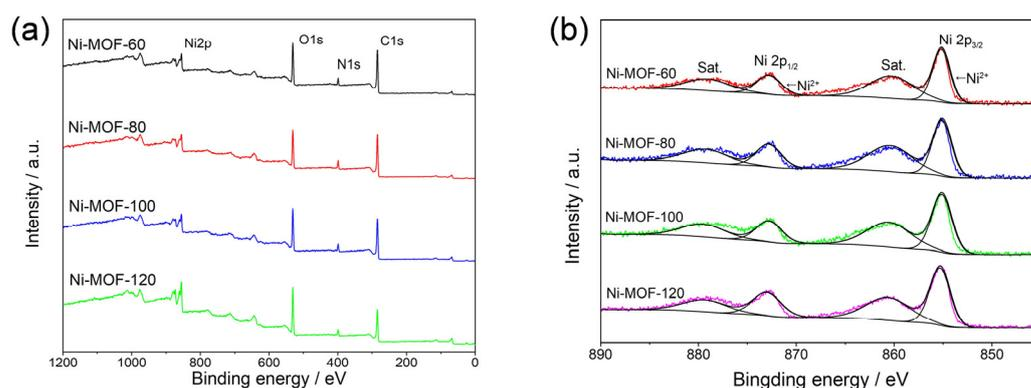
**Figure 3.** (a) Full XPS spectra and (b) Ni spectra of Ni-MOF-60, Ni-MOF-80, Ni-MOF-100, and Ni-MOF-120.
