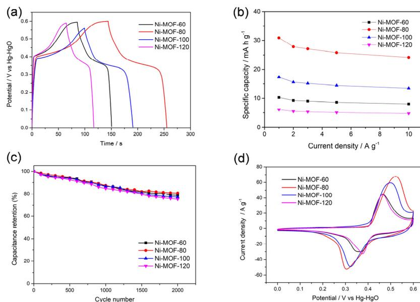
**Figure 4.** (a) GCD drawings of different Ni-MOFs at  $1 \text{ A g}^{-1}$ ; (b) Specific capacity of four samples within the range of  $1.0\text{--}10.0 \text{ A g}^{-1}$ ; (c) Capacity retention performance of four samples; (d) CV curves of different Ni-MOFs at  $100 \text{ mV s}^{-1}$ .
