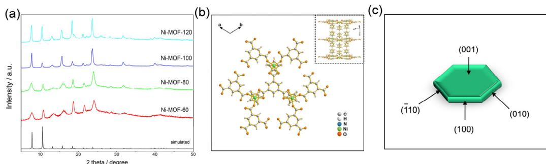
**Figure 2.** (a) X-ray diffraction patterns of Ni-MOF-60, Ni-MOF-80, Ni-MOF-100, and Ni-MOF-120; (b) Schematic diagram of Ni-MOF, Ni: green, C: gray, O: orange, and N: blue; (c) Diagram of MOF single-crystal figure.
