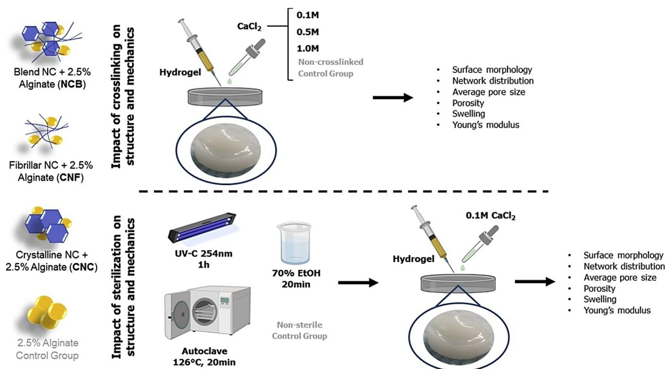
**Figure 4.** The impact of crosslinking and sterilization on mechanical and structural properties of nanocellulose-based hydrogels for cartilage tissue engineering. NCB: nanocellulose blend; CNC: nanocellulose crystals; CNF: nanocellulose fibrils. Adapted from reference [27] with permission. Copyright 2019 Elsevier.
