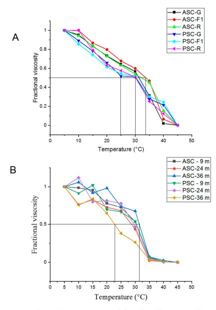
**Figure 3.** Thermal denaturation curves of tilapia skin collagen. (**A**). Collagen ASC and PSC of red, gray, and F1 strains (9-months old); (**B**). ASC and PSC collagens from F1 progeny ages 9, 24, and 36 months.
