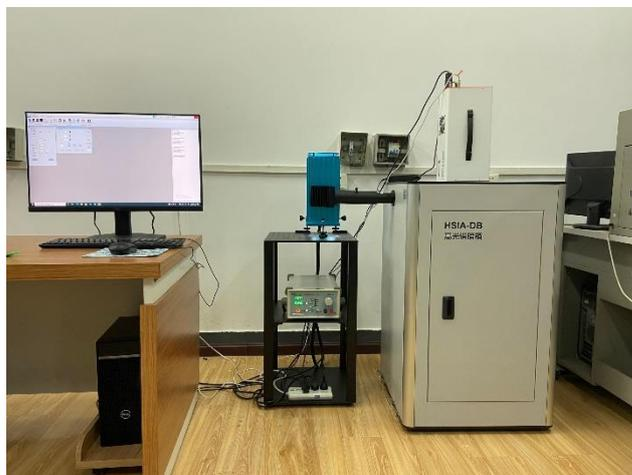
**Figure 2.** The fluorescence hyperspectral system.
