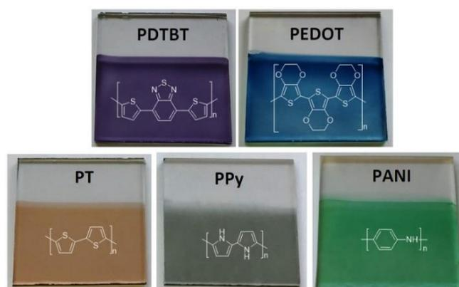
**Figure 5.** Polymer layers on FTO glass substrates obtained by oxidative electropolymerization.
