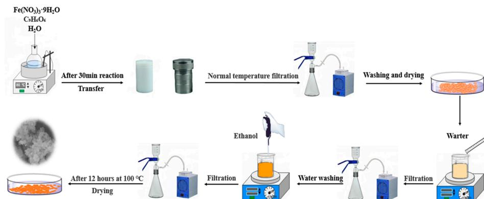
**Scheme 1.** Illustration of the preparation processes of MIL-100(Fe).
