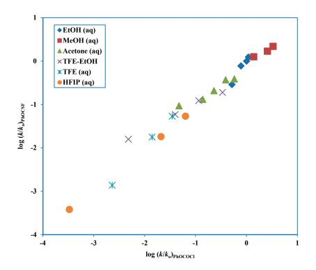
As one predicts from the enormous retardation, on replacing chlorine by fluorine, to be expected for the competing ionization pathway, a single Grunwald-Winstein correlation (for the A-E pathway) can be applied across the full range of the studied solvent compositions. Also, the  $k_{MeOH}/k_{MeOD}$  value of
